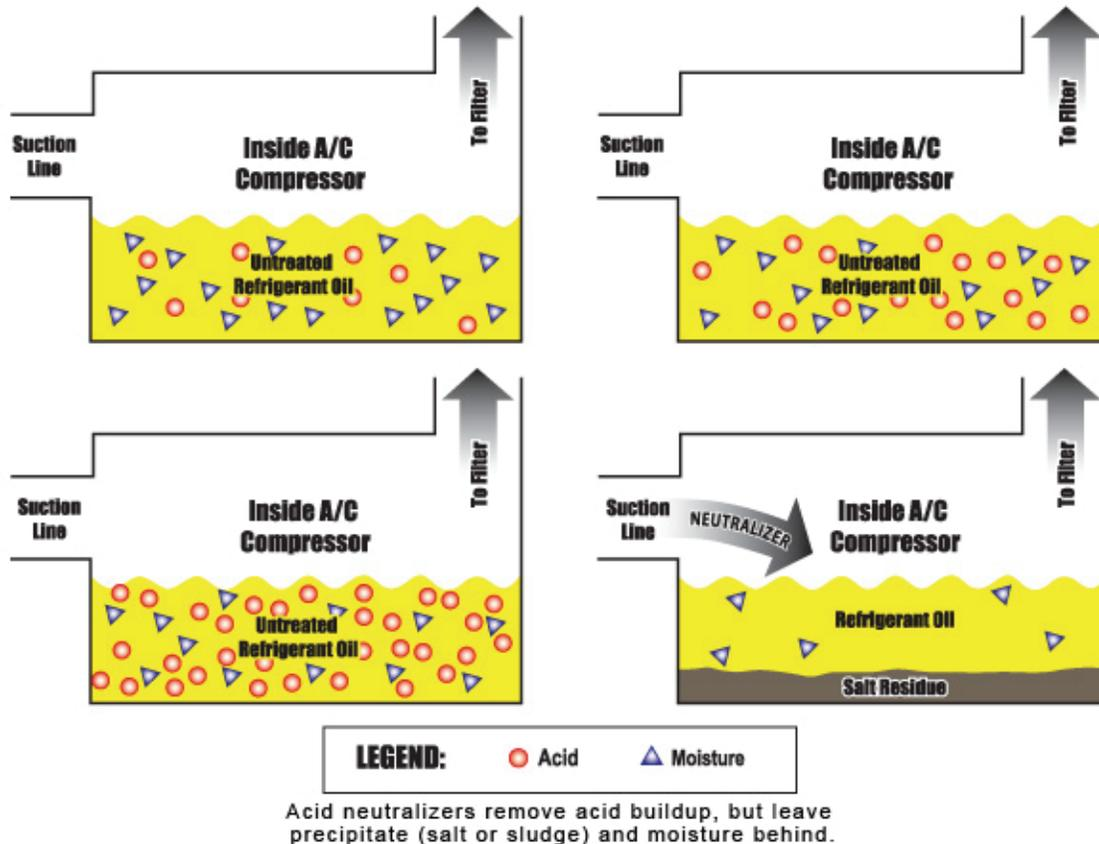
Since the new HFC systems are already plagued with sludge and water problems, potentially making more water and sludge is a really bad idea. Acid neutralizers are also less attractive in HFC/POE systems because of the many proprietary additives in the POE oil that could produce a chemical reaction that results in other byproducts - in addition to the water and sludge
