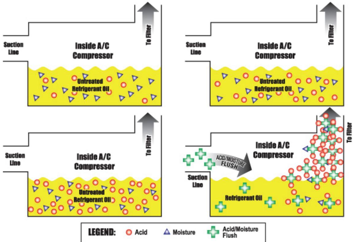
True acid removers flush both acid and water from the compressor to the filter-drier, leaving no harmful sludge inside the system.
