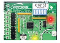
If the **Yellow** LED is off, verify power to the Qwik**Swap® V3** board. If the **RED** LED is off or flashing, there is a communication error.
