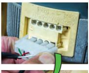
4-pin Connector from Motor to Qwik**Swap® V3** Board
