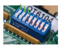
In this figure the motor has been set to 1/3 hp: (ON, ON, ON, OFF, OFF, OFF, OFF)
