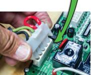
5-pin Connector from Motor to Qwik**Swap® V3** Board
