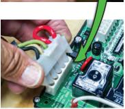
5-pin Connector from Motor to Qwik**Swap® V3** Board then...
