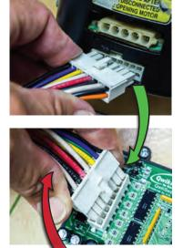
16-pin Connector from Motor to Qwik**Swap® V3** Board
