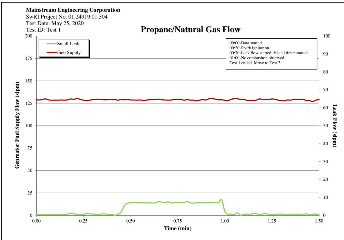
**Figure C-4. Test 1: Gas Flow Rates.**
