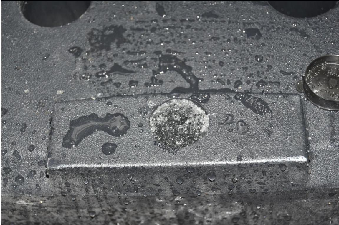
**Figure D-3. View of *QwikHurricane*<sup>®</sup> Generator Pad<sup>™</sup> Filled Prior to Testing.**
