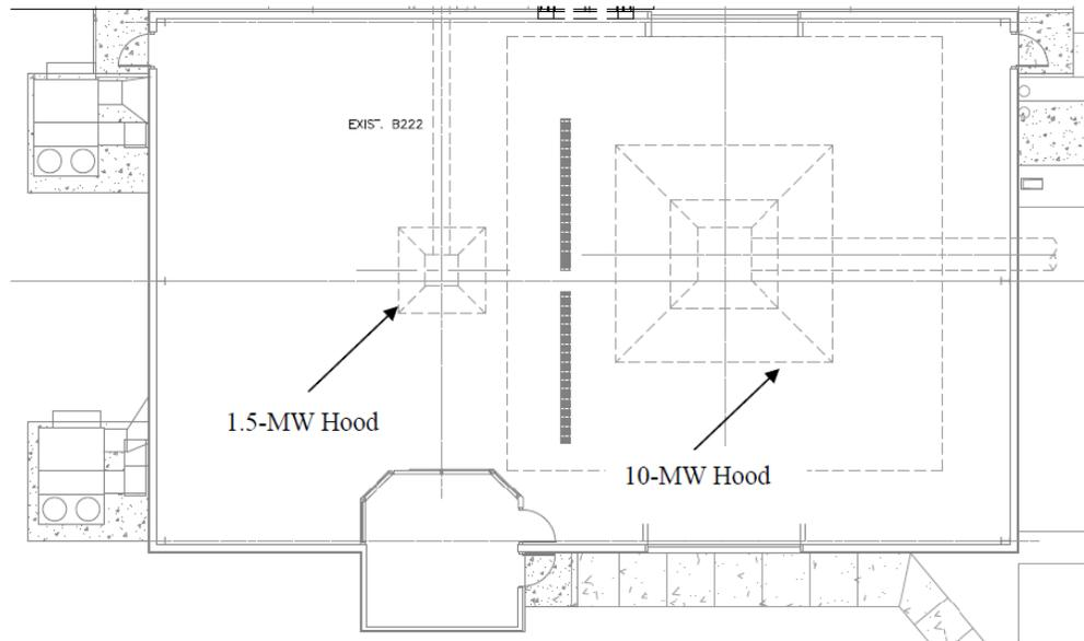
**Figure 2. Plan View Schematic of SwRI's Calorimetry Test Facility.**
