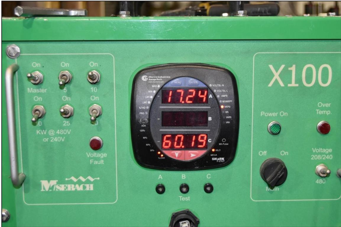
Figure D-5. Electrical Load for Generator during Warmup Period.
