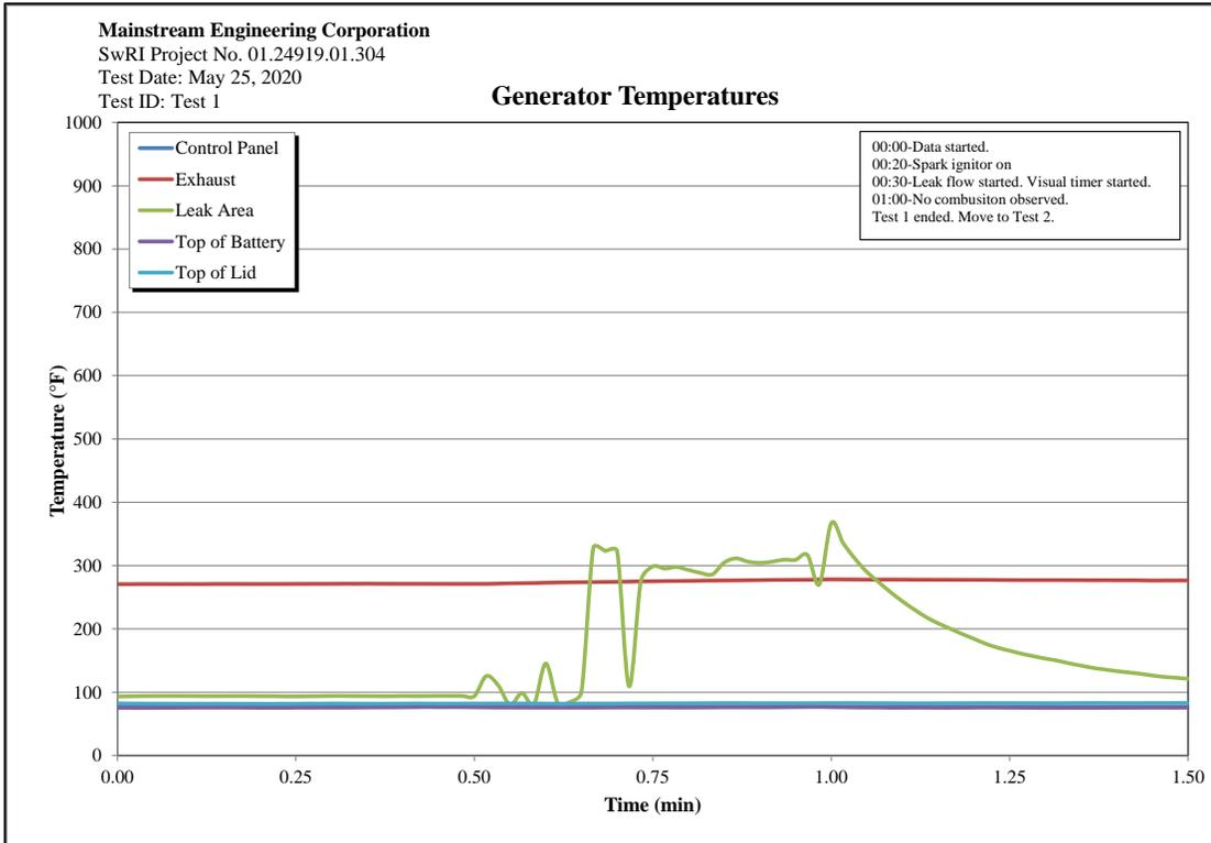
**Figure C-1. Test 1: Generator Temperatures.**
