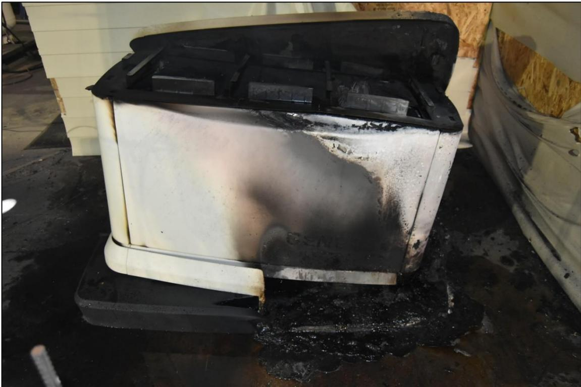
**Figure D-10. View of Generator and Pad after Test 2.**
