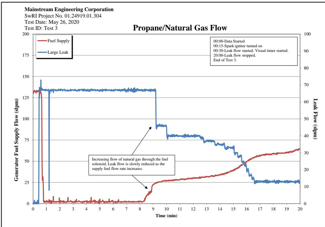
**Figure C-12. Test 3: Gas Flow Rates.**
