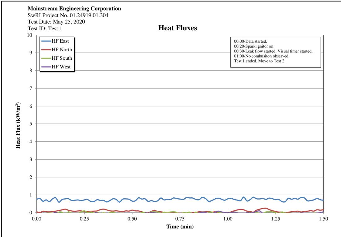
**Figure C-3. Test 1: Heat Flux Measurements.**
