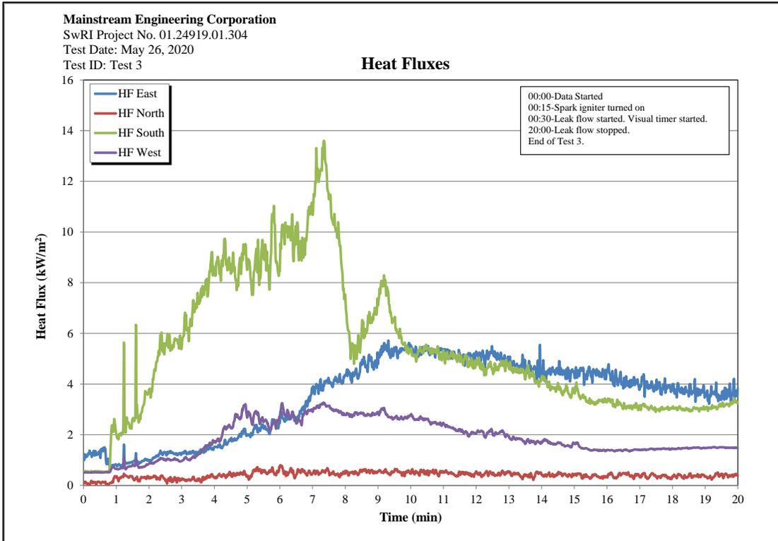
**Figure C-11. Test 3: Heat Flux Measurements.**
