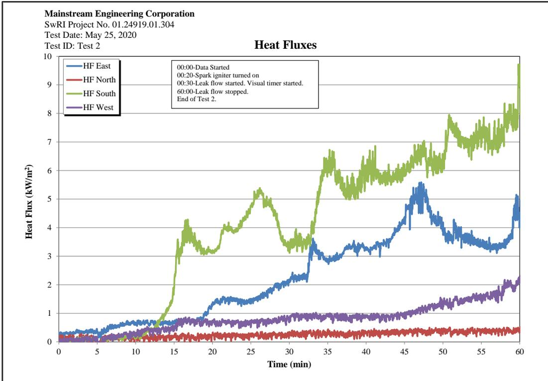
**Figure C-7. Test 2: Heat Flux Measurements.**
