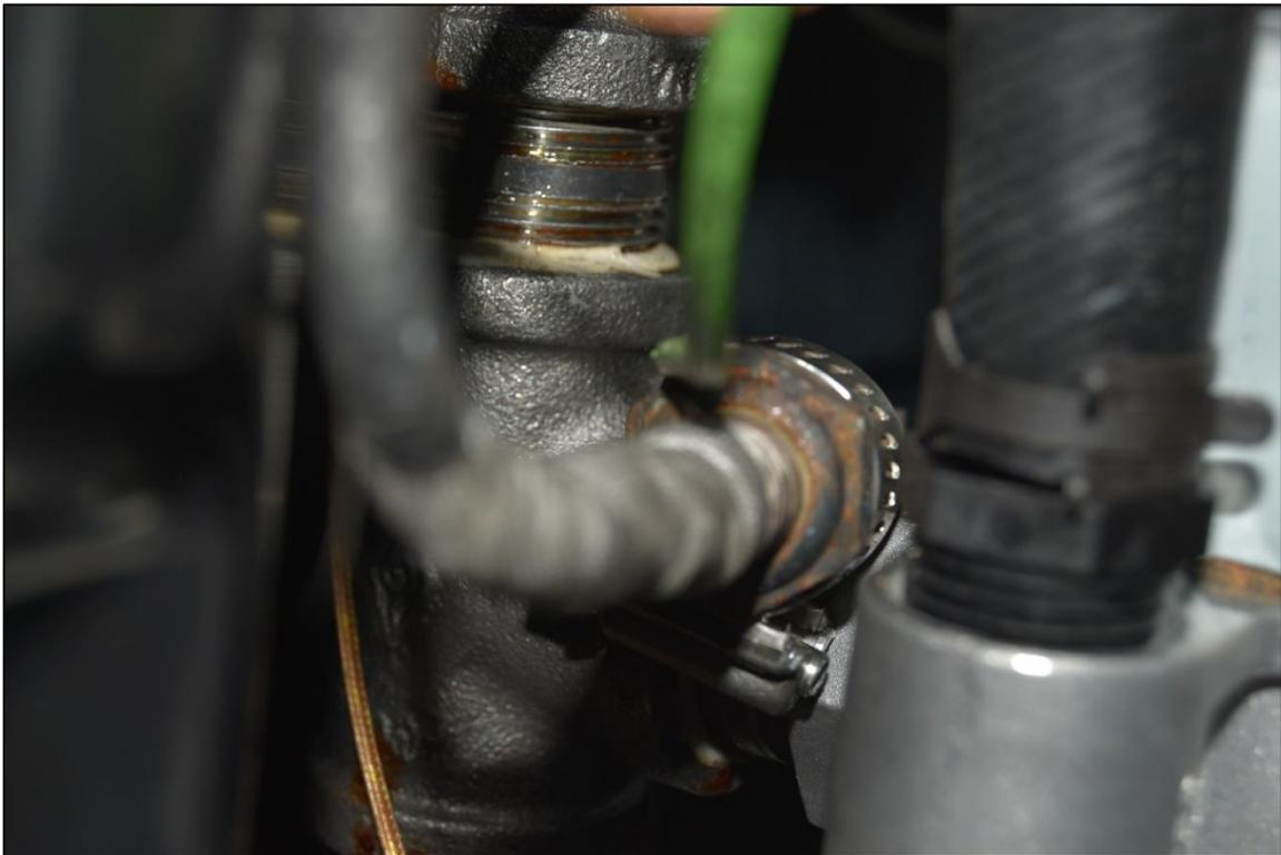
**Figure D-12. View of Spark Igniter and Leak Location for Test 3.**
