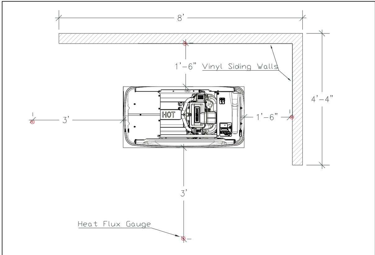
**Figure 3. Plan View of Test Setup Stand-off Distances.**
