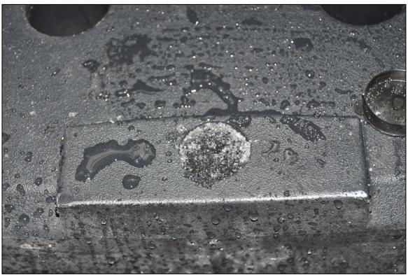
Figure D-3. View of  $QwikHurricane^{\otimes}$  Generator Pad<sup>TM</sup> Filled Prior to Testing.
